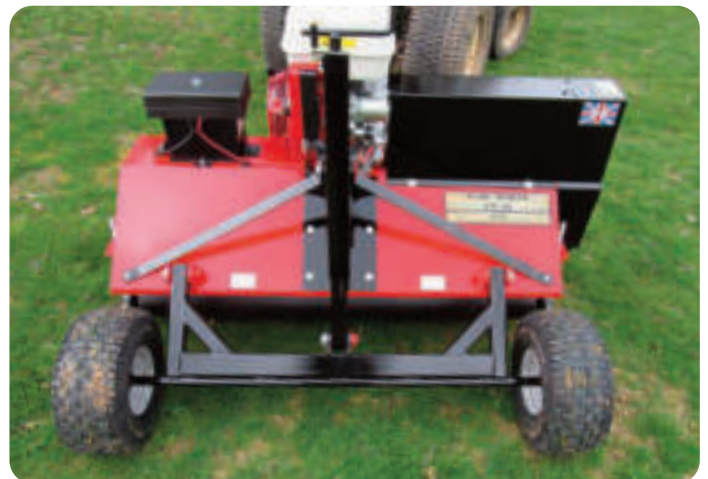
Above: The FM48's heavier 13HP engine is mounted centrally for more stable weight distribution.
