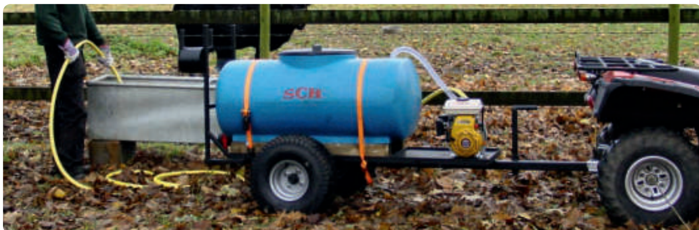
Above: ADMD with Large Flotation Wheels & 1" Petrol Pump
