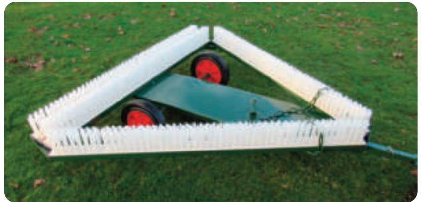
Above: TMB2 in the transport position, towed via the hitch for balance.
