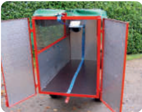
Above: Secure the blue strap inside the TRCL before collecting the debris.
