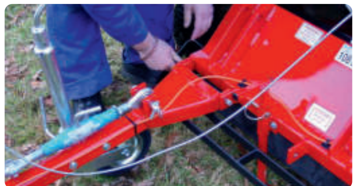
The tow bar has two operating positions, one in the centre of the machine and the other to one side where it is beneficial not to run on the standing growth before cutting.
