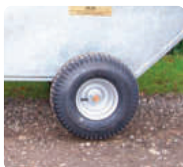
Above: 16/650x8 Wheels for GDTT/GALV & GT/GALV
