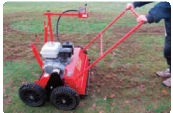
The RR3 pulling thatch and moss to the surface.
