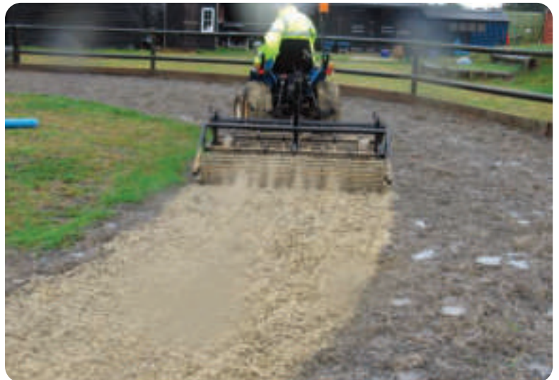
Above: The MSMGT60 rejuvenating a sand & fibre manege.
