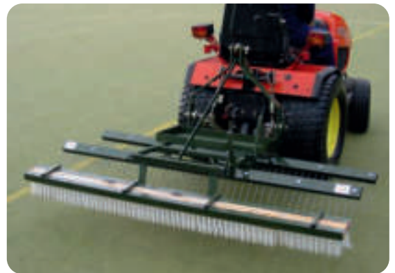
The 60" 3ASR2 attached via a 3-point Linkage
