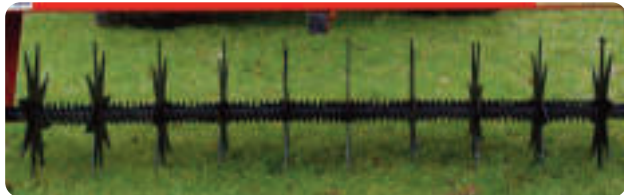
Left: Springs between Slitler Stars to protect them from damage.
