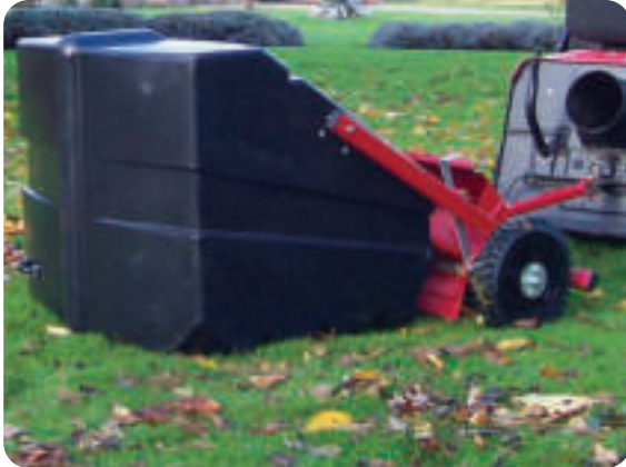
Powered by the forward speed of the towing vehicle
