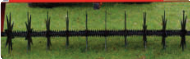
Left: Springs between Slitter Stars to protect them from damage.
