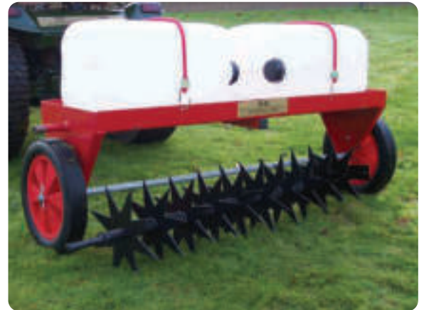
Slitter attachment in front of the Carrier Frame
