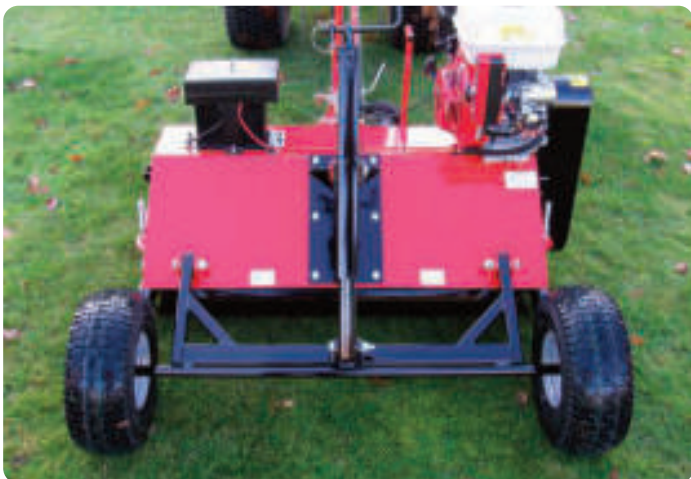
Above: The FM42's 9HP engine is mounted on the side.
