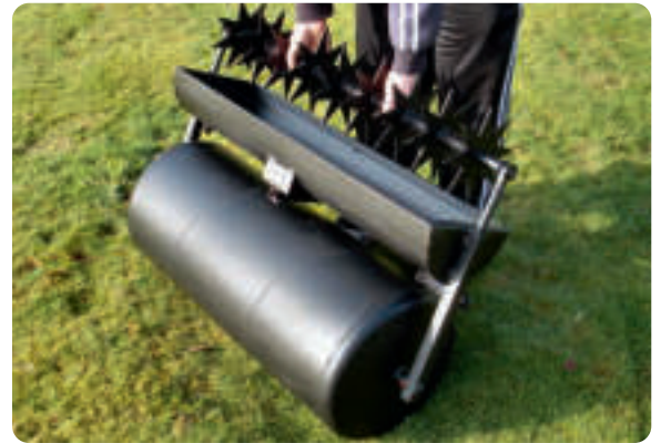
Slitter attachment being fitted
