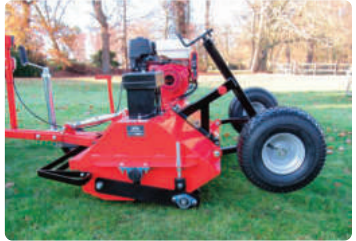
Above: The FM42 resting on the rear anti-scalping roller.
