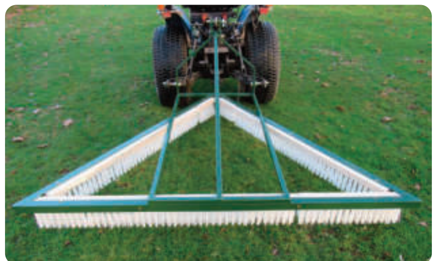
Above: 3TMB2 attached via a 3-Point Linkage.
