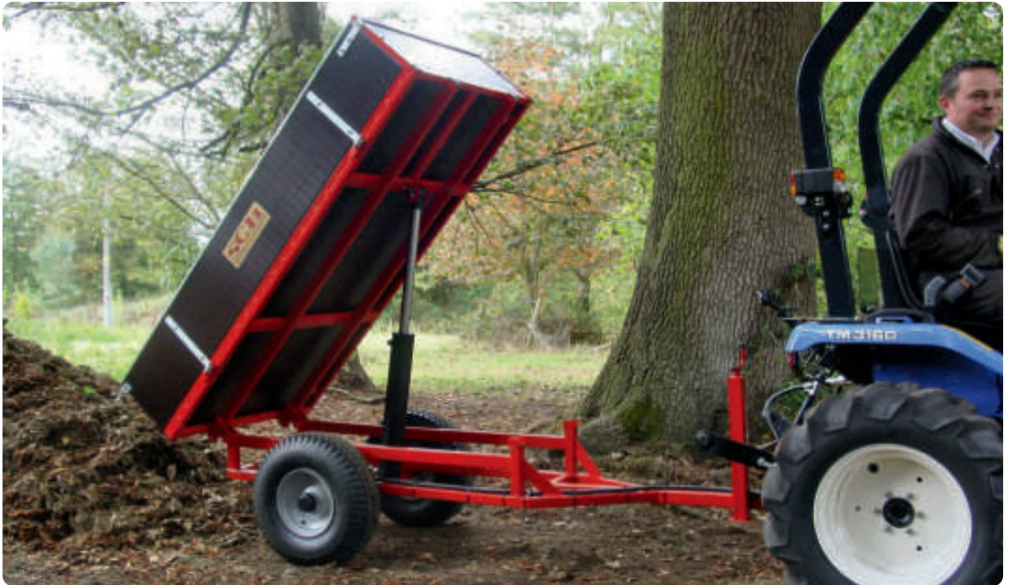
Above: HTRL1 tipping with hydraulics powered by a single acting spool (Tractor 1 Pipe)
