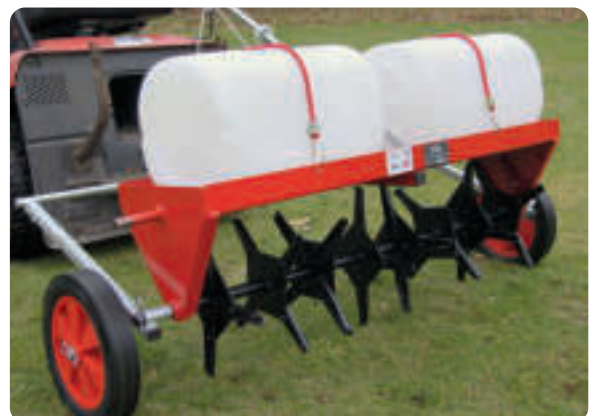
Hollow Tine Corer being lifted by the HGL.
