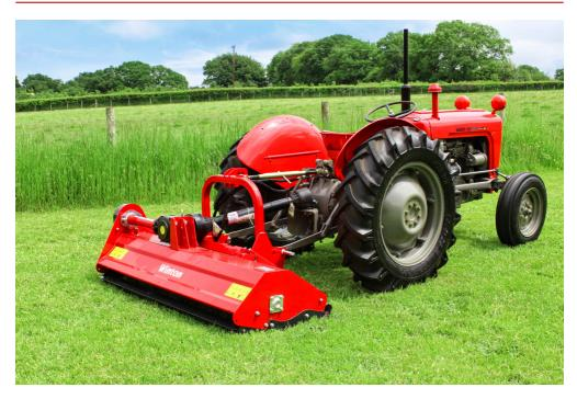
These flail mowers share the same specifications as the WFL range with the addition of the ability to offset the postion of the mower. This is achieved through the hydraulic spools of the tractors. Requires one double-acting hydraulic spool to operate.
