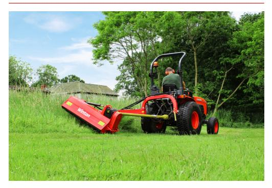
Hydraulically operated offset and cutting-head tilting function. Perfect for cutting verges, ditches and low hedges. Requires two double-acting hydraulic spools to operate.
