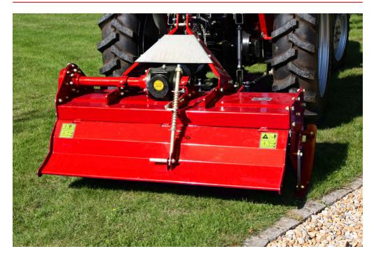
Heavy-duty machine ideal for tilling and breaking up compacted ground. The skids are height-adjustable for flexible use. The rear flap can be used to create a smooth, level finish to the soil.
