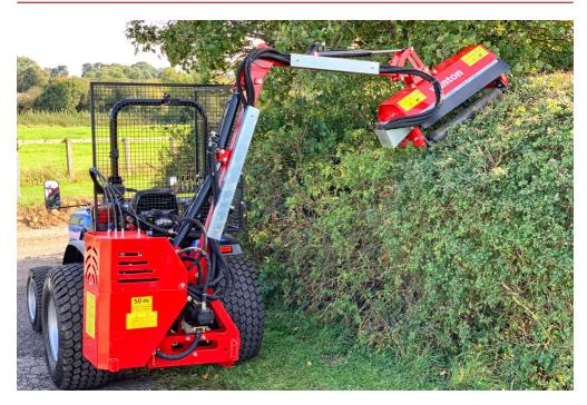
The fully adjustable cutting arm makes these machines very versatile. Fitted with Y-style flail blades and a PTO-driven hydraulic pump. The hedge cutter does not require hydraulic spools to operate. Recommended for tractors with a cab or safety mesh and suitable weights.
