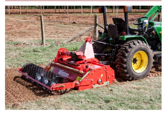
Rotovates the soil and buries small stones, debris and weeds whilst levelling the ground for a smooth new seedbed. The heavier stones and debris are placed underneath the lighter tilled soil which then lays on top ready for seeding.
