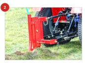
Lower the ripper into the ground whilst moving the tractor forward slowly. The tractor should be in low-range gear 1 or 2.
