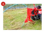
When finished or at the end of a row, lift the ripper and cut pipe to size as required.
