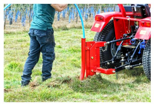
Ideal for laying water pipe or armoured cable around paddocks. The ripper can physically go down 24 inches, but the achieved depth depends on the tractor and soil type.
