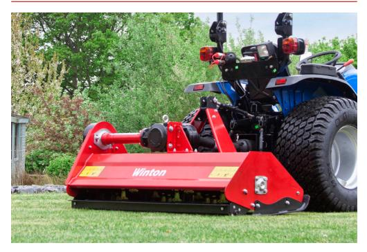
Heavy-duty design makes these flail mowers great all-rounders for a wide range of applications. The heavy hammer blades are suitable for long grass and heavier scrub materials. Flail blades mulch up the grass cuttings and give a close cut.
