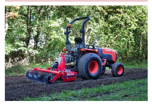
Designed for less stony/rocky areas with no grass. Ideal for aerating the ground and enabling the soil to gain warmth quicker so that planted materials can grow in healthier conditions.
