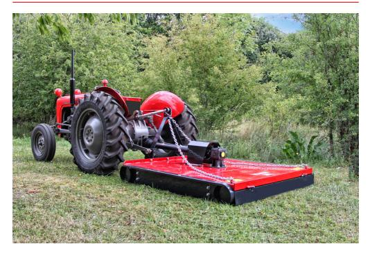
Perfect for paddock maintenance and cutting overgrown grass, weeds, light scrub and saplings. Direct drive to suit lower-horsepower tractors. Rotary blades slice the 'top' off grass and weeds.
