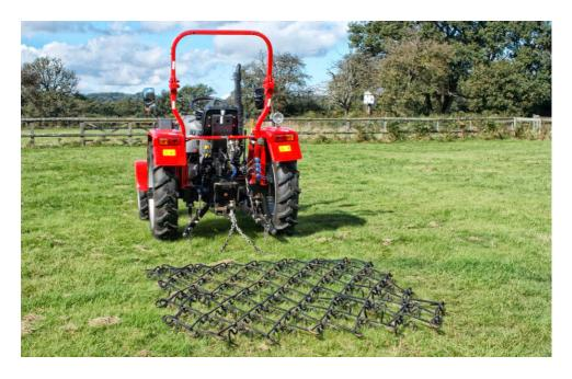
These framed harrows are ideal for use around smallholdings and paddocks. They can be folded to fit through gateways and for storage and attaches to a tractor linkage for moving between fields. The 3-way harrow tines give an aggressive harrow, then a slightly less vigorous harrow when spun around and finally a light harrowing when upturned.
