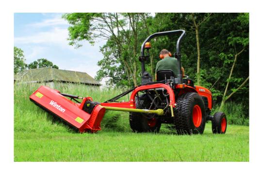
Winton flail hedge cutters are great for cutting hedges, ditches, embankments and roadsides. Fitted with Y-style blades and a PTO-driven hydraulic pump, which means the attachment is independent of the tractor's hydraulics. The fully adjustable arm make these machines very versatile. Great pieces of equipment for estates, smallholdings or paddocks.
