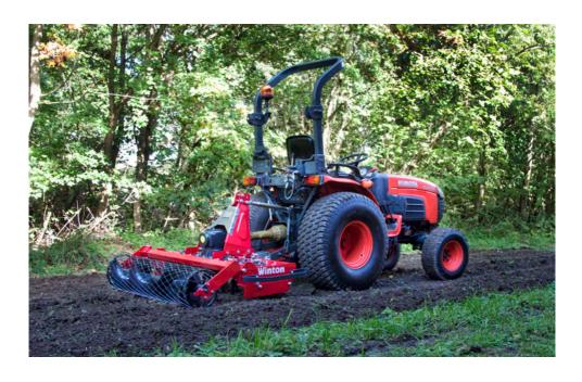
Rotary tillers are ideal for tilling and levelling the ground. These machines break up compacted soil on allotments ready for planting. Skids are height adjustable for flexible use and rear flap creates a smooth level finish to the tilled soil.
