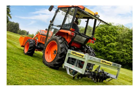
The ripper and pipe layer is ideal for laying water pipe or armoured cable. The attachment benefits from being both quick and easy to use.
