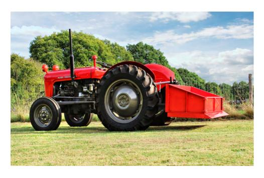
Box grader blades are designed for levelling ground and tracks. The height-adjustable ripper tines are perfect for ripping the soil to a variety of depths. Alternatively the tines can be set at the highest point or removed to use the implement as a grader blade.
